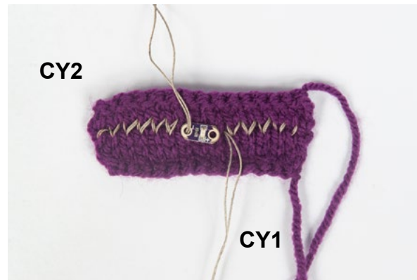
Figure 32: Front view of the belt (flipped horizontally). CY1 is now on the right and CY2 is on the left. The LED is positioned with the negative tab threaded, ready to be sewn in place.
