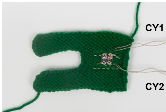
Figure 43: LEDs are sewn in place between the CY rails with positive tabs attached to CY1 (top rail) and negative tabs to CY2 (bottom rail).
