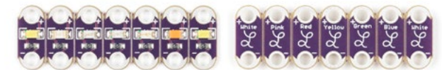
Figure 3: A strip of Rainbow LEDs, front and back. In this strip the LED colours are written on the back and include two LilyPad white LEDs and one pink, red, yellow, green and blue LED.
