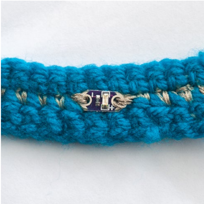
Figure 12: LED tabs secured with conductive yarn.
