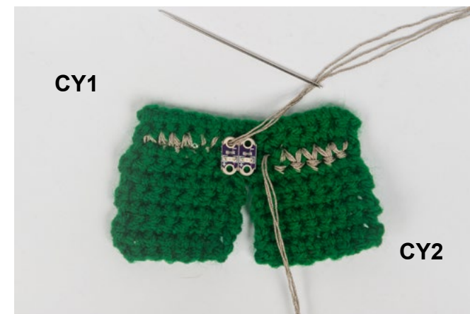
Figure 68: With the remaining CY tails threaded through to the front of the shorts, the CY1 tail strands are then threaded through the negative tab of the first of two LEDs to sew in place.
