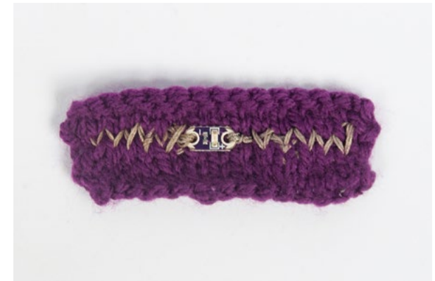
Figure 33: Front view of the completed belt with the LED's negative (-) tab to the left and positive (+) to the right.
