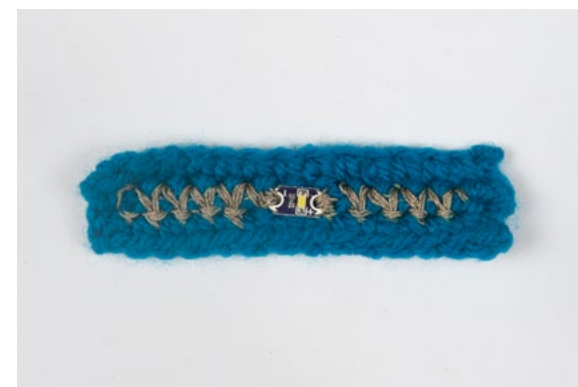
Figure 64: Front view of the completed belt with the LED's negative (-) tab on the left and positive (+) on the right.
