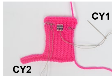
Figure 38: The remaining CY1 tail strands on the right are threaded through the negative tab of the first of two LEDs to sew in place.
