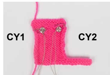
Figure 37: Both snaps are sewn in place, with the male snap on the right and female snap on the left.
