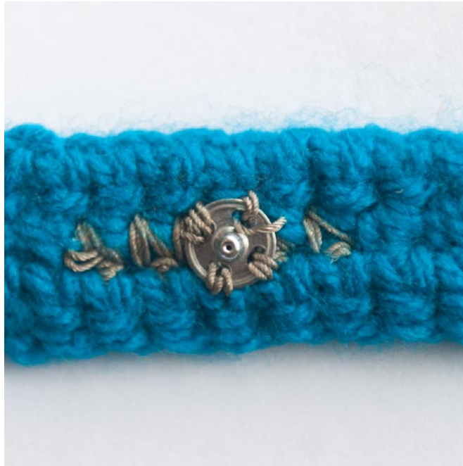
Figure 13: Male snap secured with conductive yarn.
