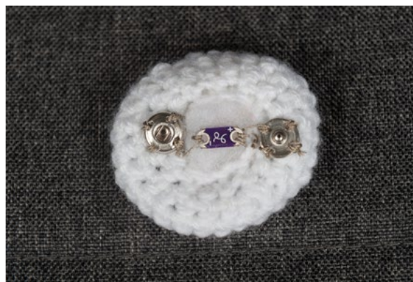
Figure 78: One CY strand was used to connect a female snap on the left to the LED's negative tab, with a second CY strand connecting a male snap to the positive tab of the LED.
