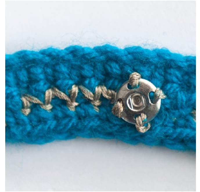
Figure 14: Female snap secured with conductive yarn.
